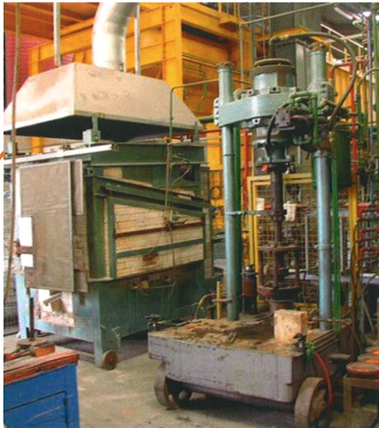
Optimisation of glass composition with pilot-scale furnaces
